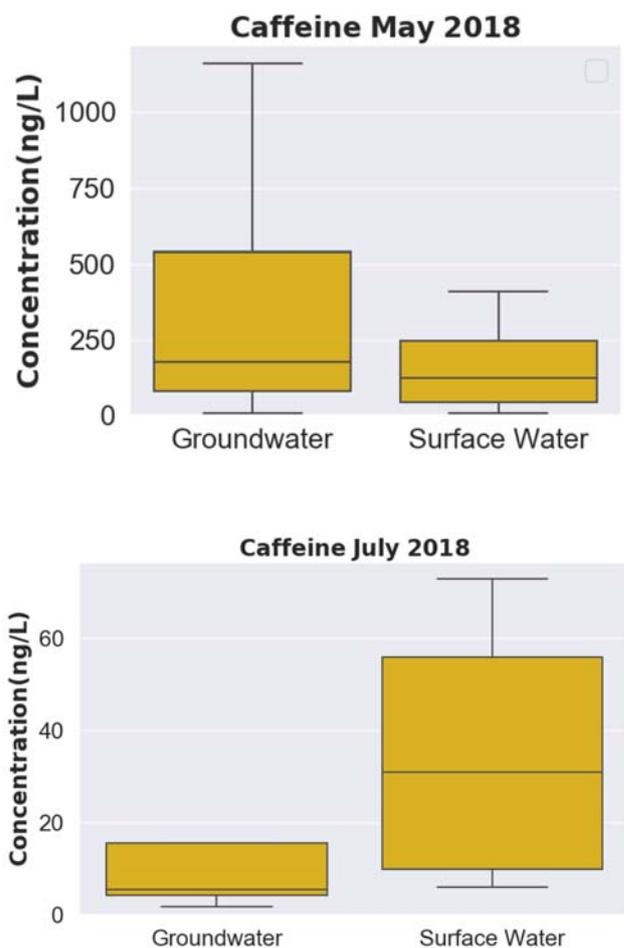
Figure 2: Concentrations of *caffeine* measured in groundwater and surface water in Fehraltorf. *Caffeine* is an indicator for untreated wastewater in the environment.
