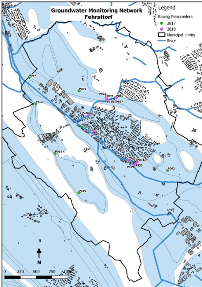
Figure 1: Shallow groundwater monitoring wells installed in Fehraltorf through the course of this study. The main body of the aquifer is shaded in light blue.
