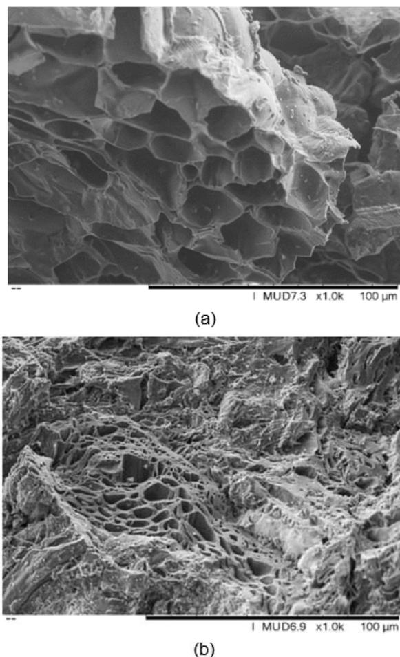
Figure 1: SEM image of biochar a) OSR550 and b) SWP550.
