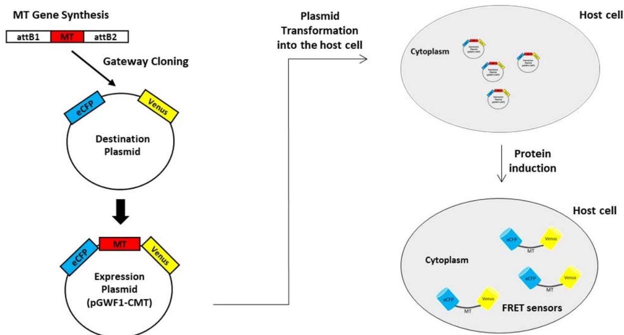
Figure 2: The stages of FRET biosensor development. A gene encoding MT was synthesised and cloned into a plasmid encoding eCFP and Venus to generate the expression plasmid (pGWF1-CMT). The pGWF1-CMT was transformed into a bacteria host cell and the FRET sensor protein production was induced by the addition of IPTG.
