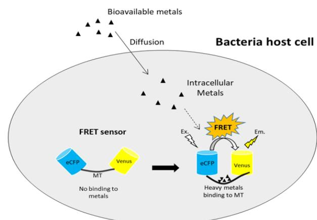
**Figure 1: Concept of biosensor: FRET sensor as a fusion of eCFP-MT-Venus protein is expressed inside the bacteria host cell. Binding of intracellular metals to MT changes the distance between eCFP and Venus. This enables FRET that can be measured by ratiometric changes in fluorescence and corresponds with metal concentrations.**
